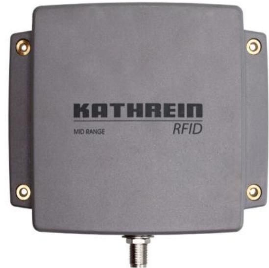
$$R_{forward} = \frac{\lambda}{4\pi} \sqrt{\frac{P_{TX} G_r G_{tag}}{P_{min,tag}}} = \frac{3 \cdot 10^8}{866.4 \cdot 10^6} \sqrt{\frac{1 \cdot 1.77 \cdot 1.31}{0.007943 \cdot 10^{-3}}} = 15,76 \text{ m}$$
