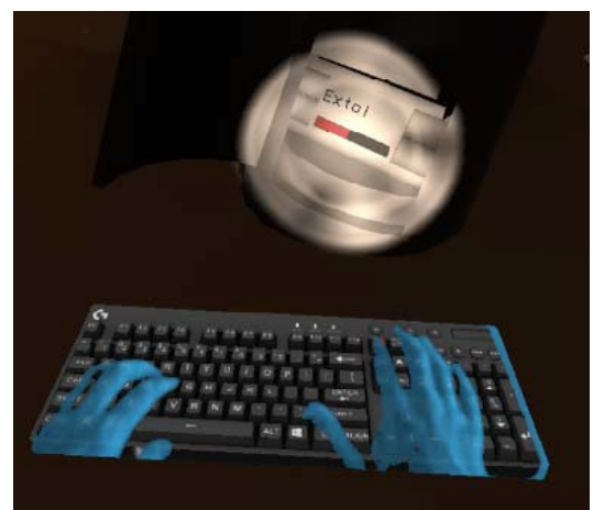
Figure 12. Logitech G810 recreated within a virtual environment with no more than the Vive's integrated camera and one Vive Tracker [Extracted from Bovet et al. (2018)]
