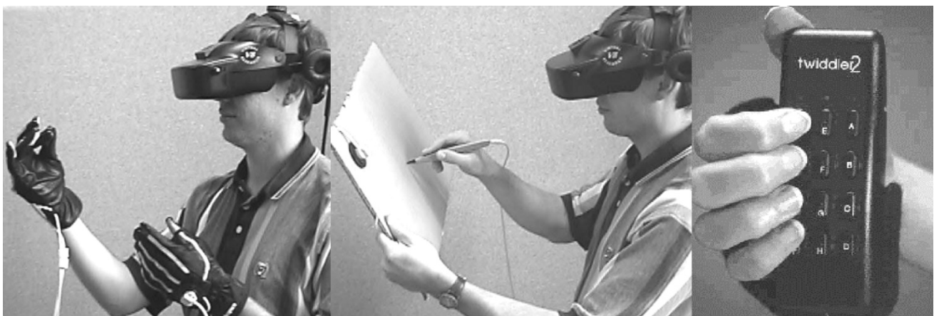
Figure 17. Specialized hardware for text input within VR [Extracted from Bowman et al. (2002)]
