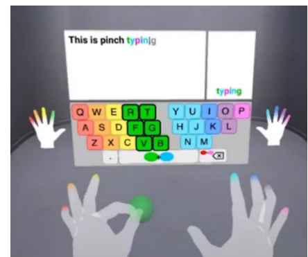
Figure 15 (Top). Touch-based keyboard concept used alongside hand tracking technology [Extracted from Markussen et al. (2013)]
