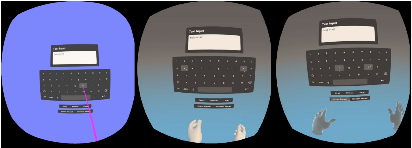
Figure 18. Oculus' single raycast approach on the left, Microsoft's dual raycast approach on the right and hand-tracking based raycasting on the right
