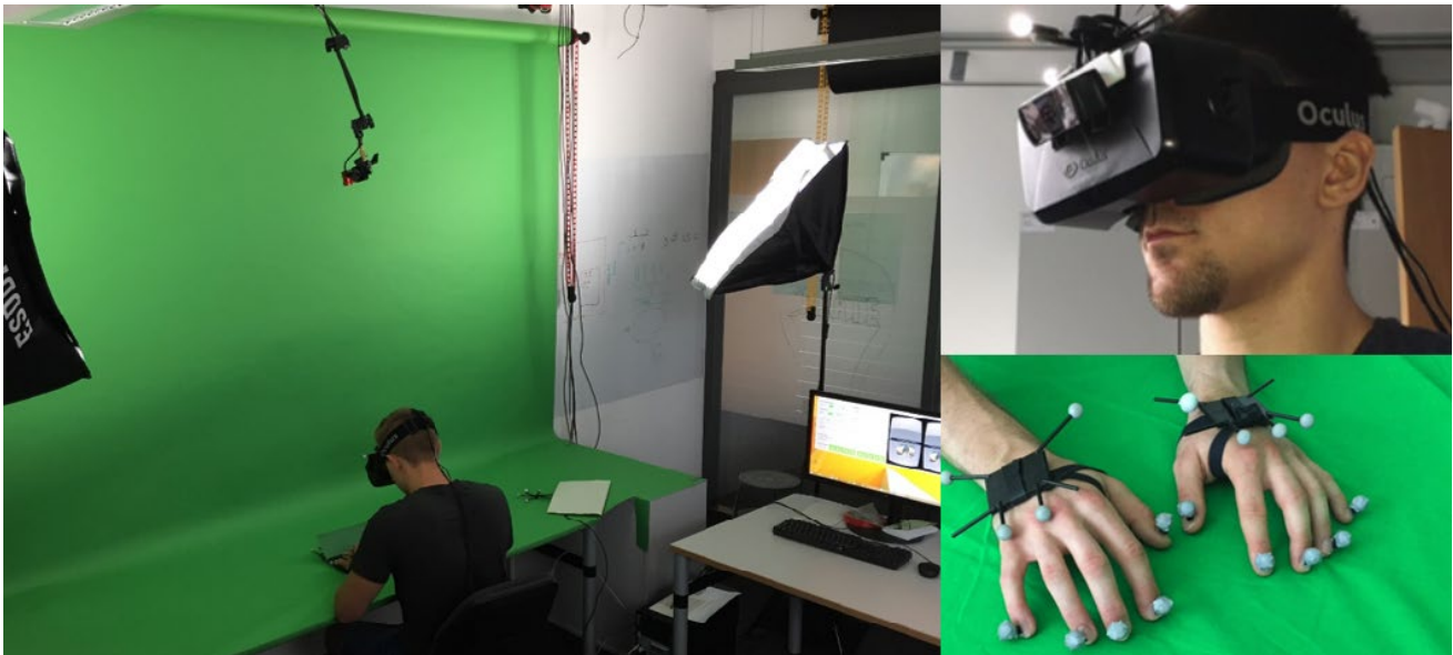
Figure 11. Grubert's chroma key compositing setup [Extracted from McGill et al. (2015)]
