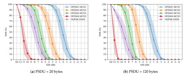
Figure 8. OFDM4-MCS5 interference results.
