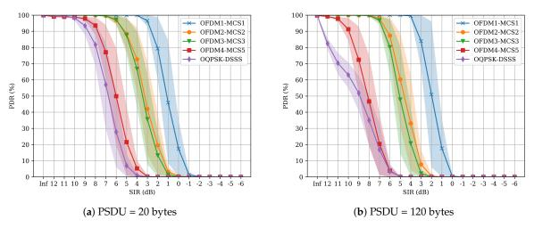
Figure 6. OFDM2-MCS2 interference results.
