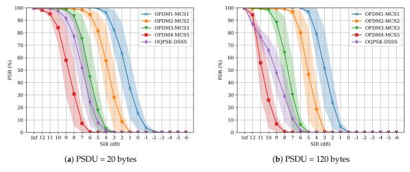
Figure 7. OFDM3-MCS3 interference results.
