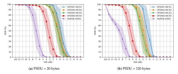
Figure 5. OFDM1-MCS1 interference results.
