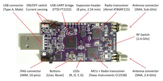
**Figure 4.** OpenMote-B board. The CC2538 (MCU) and the AT86RF215 (radio transceiver) are interconnected using the SPI bus, whereas the CC2538 (MCU) is connected to the computer using the USB-UART bridge (FTDI FT2232).
