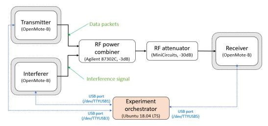
**Figure 3.** Evaluation setup. Note that the grey box around the transmitter, interferer and receiver devices represents an RF shielding enclosure used to ensure that communication between devices can only occur through the RF coaxial cables.
