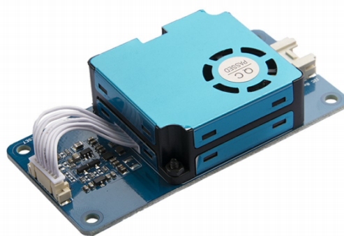
Figura 3.2: HM3001 Dust Sensor.
