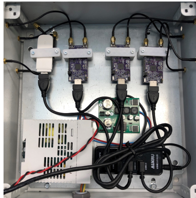
Figure 4. Gateway setup with 3× OpenMote-B boards acting as IEEE 802.15.4g SUN receivers, 1×Raspberry Pi 3B+ (not displayed), and a Huawei E3531 HSPA+ modem for Internet access.
