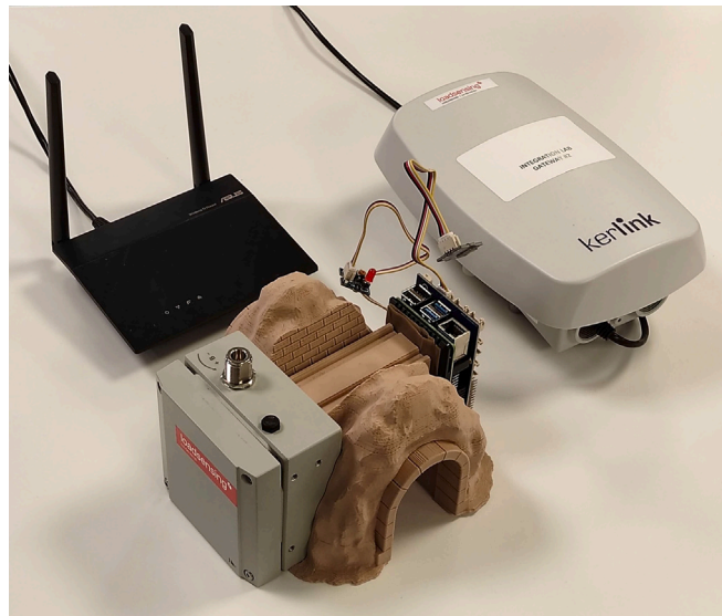
Fig. 8. Our Raspberry Pi, a Worldsensing IoT node, and two gateways.
