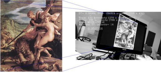
Fig. 2. Computed homography using RANSAC and keypoints and descriptors obtained with MSER/FREAK. OpenCV supports methods for matrix calculation which allows the projection of any point P from the reference image into the scene.
