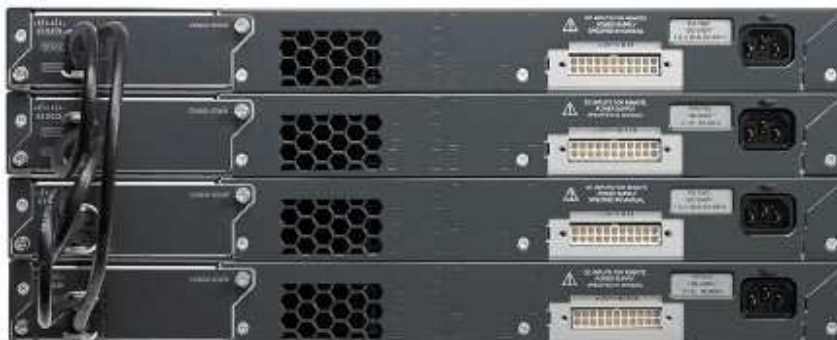
Figure 2. Cisco FlexStack-Plus Switch Stack
