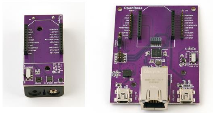
Figura 87. Mòduls OpenBattery i OpenBase per a OpenMote [30].
