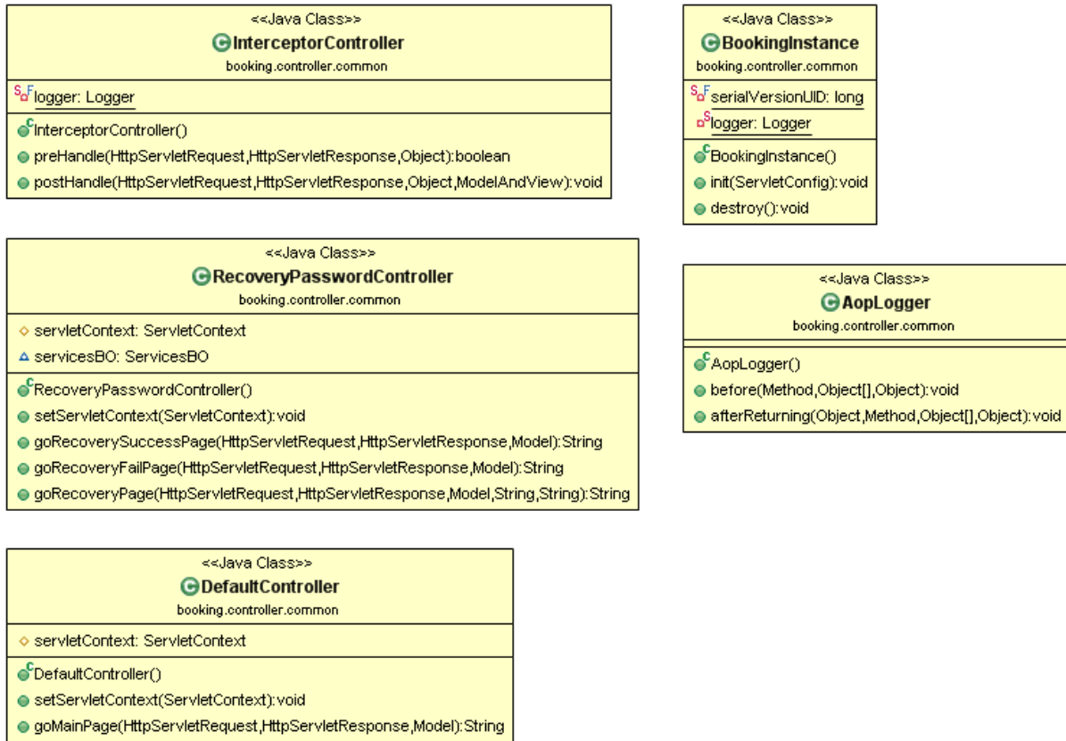
Figura 10: Diagrama de classes paquet booking.controller.common
