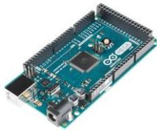
Figura 21: Arduino Mega 2560
