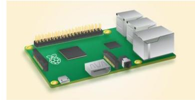
Figura 20: Raspberry Pi 2 Model B
