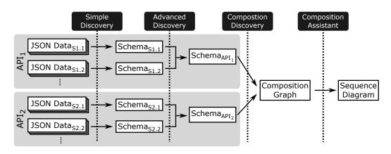
Figure 1: Discovery of the implicit structure from a set of JSON-based Web APIs. The main functionalities of our tool are represented with black-filled rounded boxes while input/output data is depicted as white-filled boxes.
