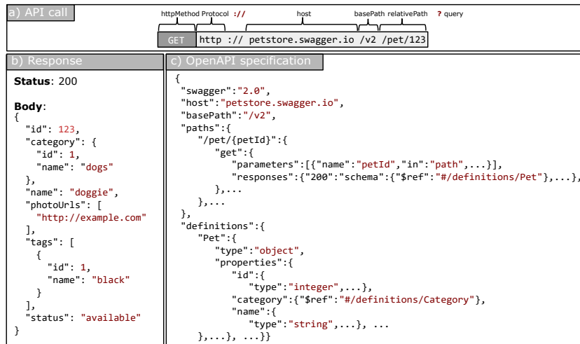
Fig. 1. API call example of the Petstore API: (a) the request, (b) the response, and (c) an excerpt of the corresponding OpenAPI specification.
