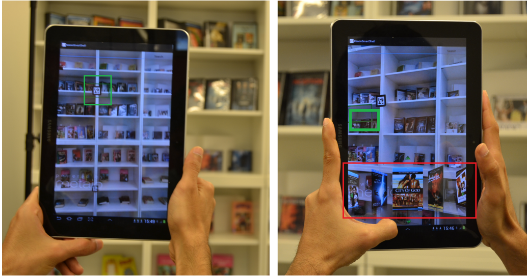
Figure 5: (A) Hand-held device pointing at the smart shelf, where the AR marker is visible. (B) Close up view of the hand-held screen, showing the superimposed item information, and the green square indicating the active area, i.e. the user clicked location.
