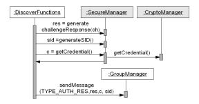
Figure 4: (Broker) Authentication sequence diagram: authRequest function.
