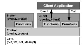
Figure 1: JXTA-Overlay architecture.
