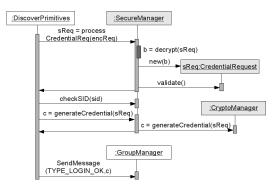
Figure 7: (Broker) Login sequence diagram: secureLogin function.
