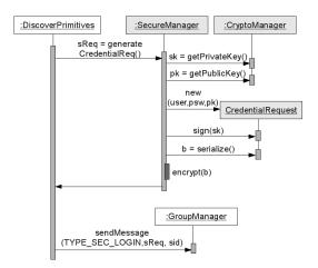
Figure 6: (Client) Login sequence diagram: secureLogin primitive.
