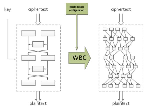
Figure 4.1: Basic idea behind the term White-Box Cryptography [SOF12].
