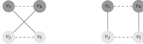
Fig. 2: Valid swap operation among vertices v_i, v_j, v_k and v_l . Dashed lines represent deleted edges while solid lines are the added ones.
