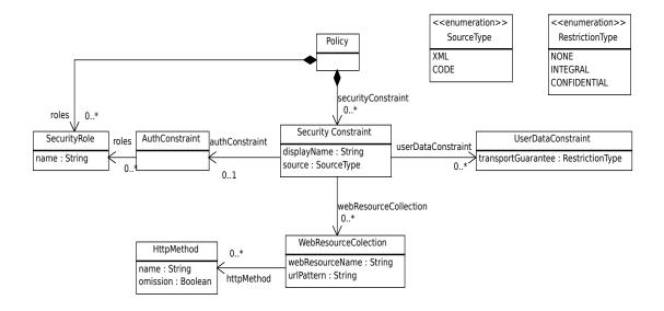
Figure 13: Servlet Security metamodel
