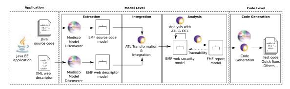
Figure 17: Architecture of our Java EE web application analysis approach
