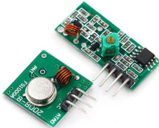
FIGURA 21 - EMISOR Y RECEPTOR DE 433 MHZ
