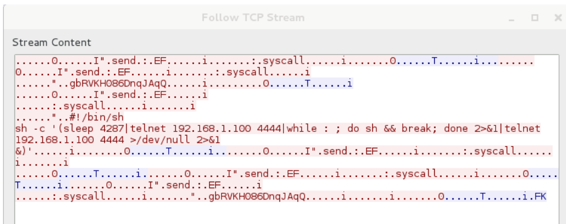
Figura 5.18: Captura Wireshark, detalle paquete, Exploit exploit/linux/misc/dr_b_remote_codeexec
