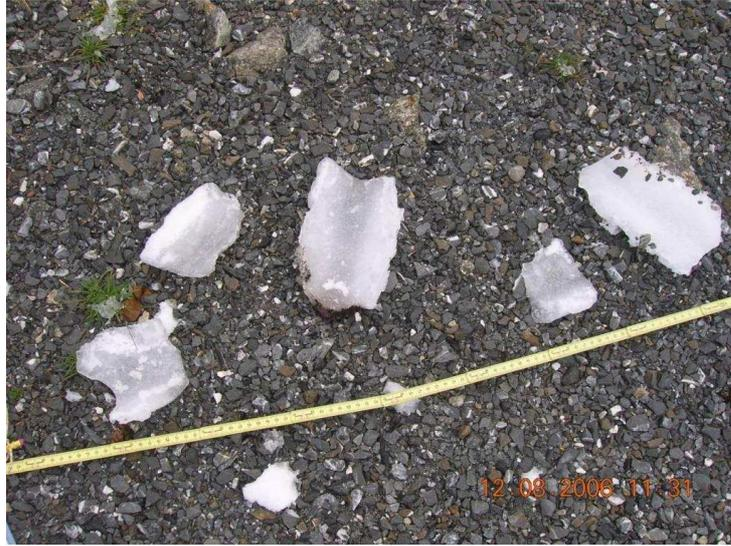
Figure 6.15: Pieces of ice thrown from a HAWT turbine blade. Photo credit: Alpine Test Site Güttsch, Federal Office of Meteorology and Climatology, Switzerland.
