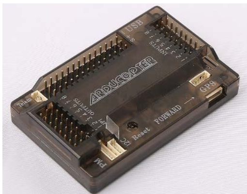
Figura. 16 Arduino APM Copter 2.6 (ArduCopter)
