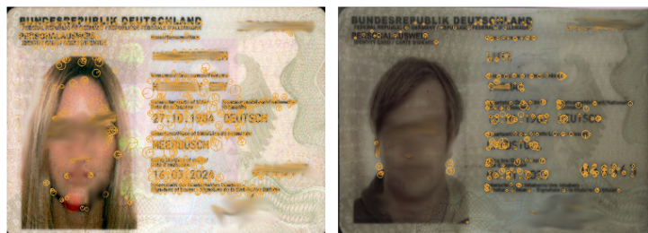
Figure 26. Effects of low contrast in feature extractors: we lost several key points.
