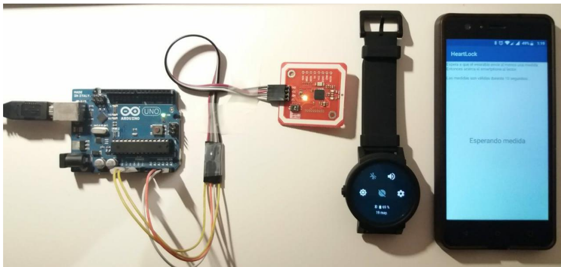
Figura 26. Escenario completo (Arduino UNO, PN532, wearable Wear OS, smartphone Android).
