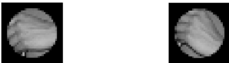
Figure 3: Applying a circular mask to the windows on both original image (left) and the rotated version (right) the information shown is now practically identical.
