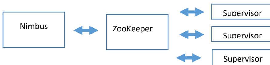
Figure 1: Nodes Interaction between the Nimbus, Supervisor and Zookeeper
