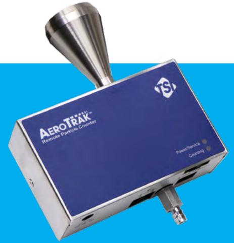
The TSI AeroTrak® 7201, 7301 and 7501 Remote Particle Counters offer the most features and flexibility out of any remote particle counter on the market today. Integration is easy using either Ethernet (TCP/IP) or serial Modbus RTU communications. The instrument can be powered over its Ethernet connection (Power-over-Ethernet) to simplify installation, or via a local power supply. Configuration can be done locally with a PC or via a web browser.
