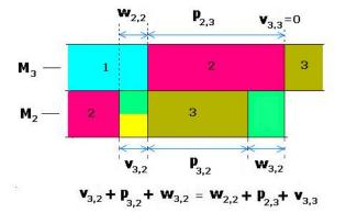
Fig. 2. Flow conservation constraint for job i = 2 and machine k = 2.
