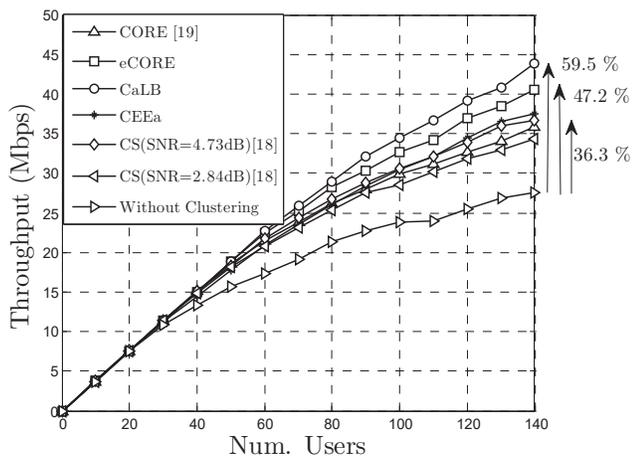
Fig. 3. Downlink throughput for the set of algorithms.
