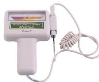
FIGURA 6. SENSOR CLORO Y PH [41]
