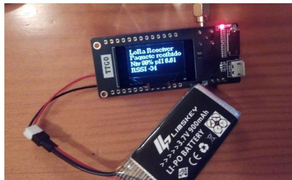
FIGURA 46. PRUEBA\_UNO TTGO RECEPTOR
