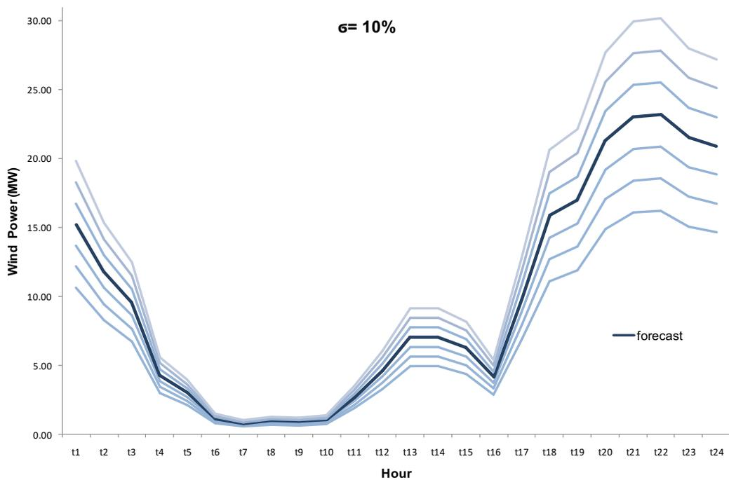
**Figure 4-2** Wind power forecast and the generated scenarios at 24-h, with  $\sigma=10\%$
