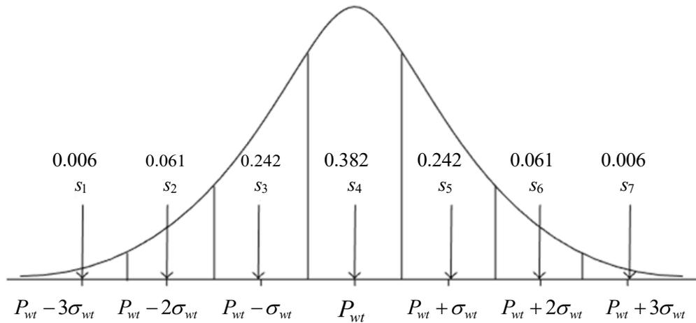
**Figure 2-3 Seven-interval discretization of a normal distribution, No. of standard deviations from the mean (s4). Mean= forecast**
