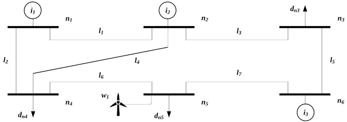
Figure 2-2 Power system diagram – 6 buses system example
