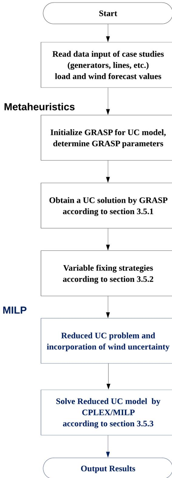
Figure 3-1 Flowchart proposed matheuristics approach to solving the UC model
