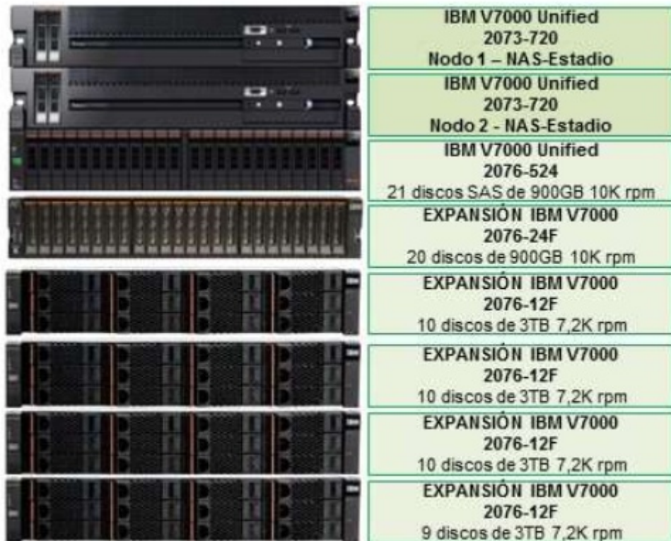
Figura 8 - Cabina de disco IBM Storwize V7000 Gen 2 Unified.
