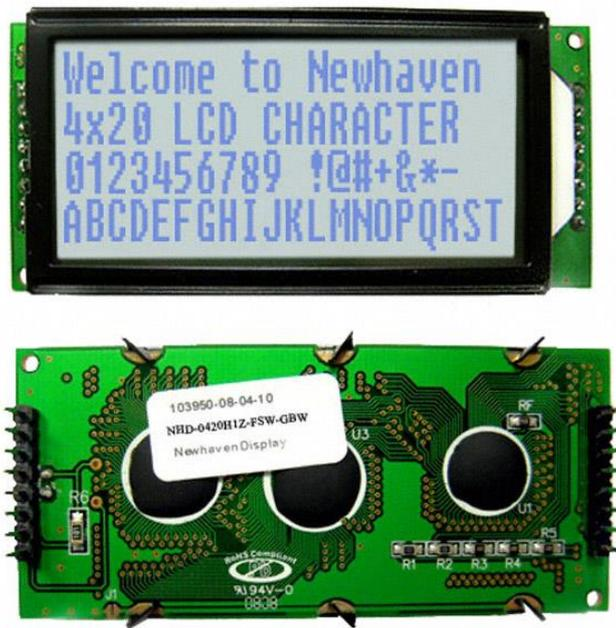
*Figura 38 Display LCD 4x20 [18]*
