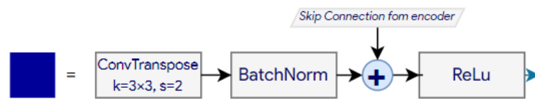
Figure 5.15: Decoder building block for Skip connection CAE.
