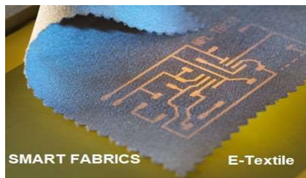
Figura 2: Circuit integrat en el teixit. Font: Topic for seminar (2018) Smart and Electronic Fabric. Seminar Report. https://www.topicsforseminar.com/2018/04/electronic-textile-seminar-report.html
