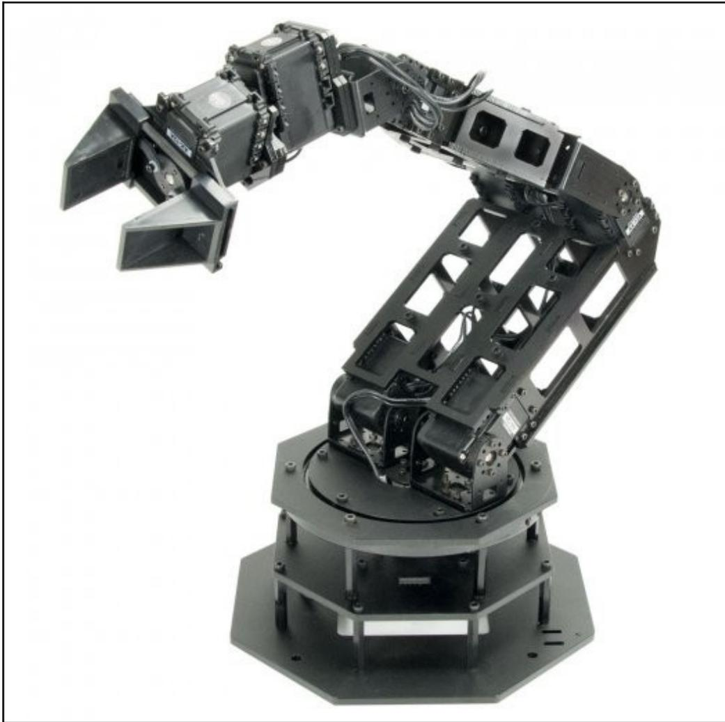
Figura 7. PhantomX Reactor Robot Arm
