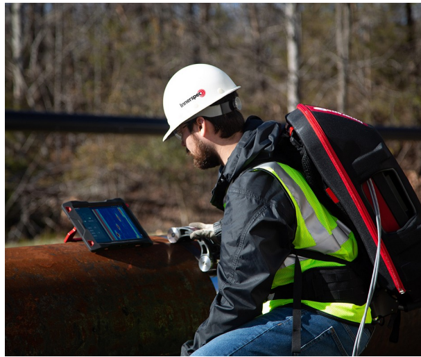
Figure 1: NDT professional inspecting corrosion in a pipe using an Innerspec instrument
