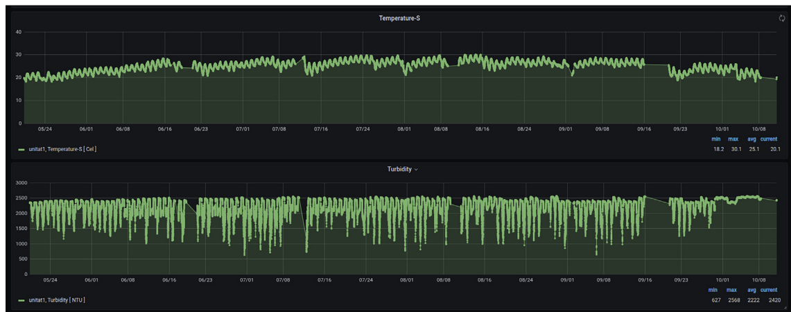
Fig. 10. Temperature and turbidity data collected from June to October 2021, with a sampling rate of 2 min. Data show daily patterns influenced by the repetitive activities in the pond.
