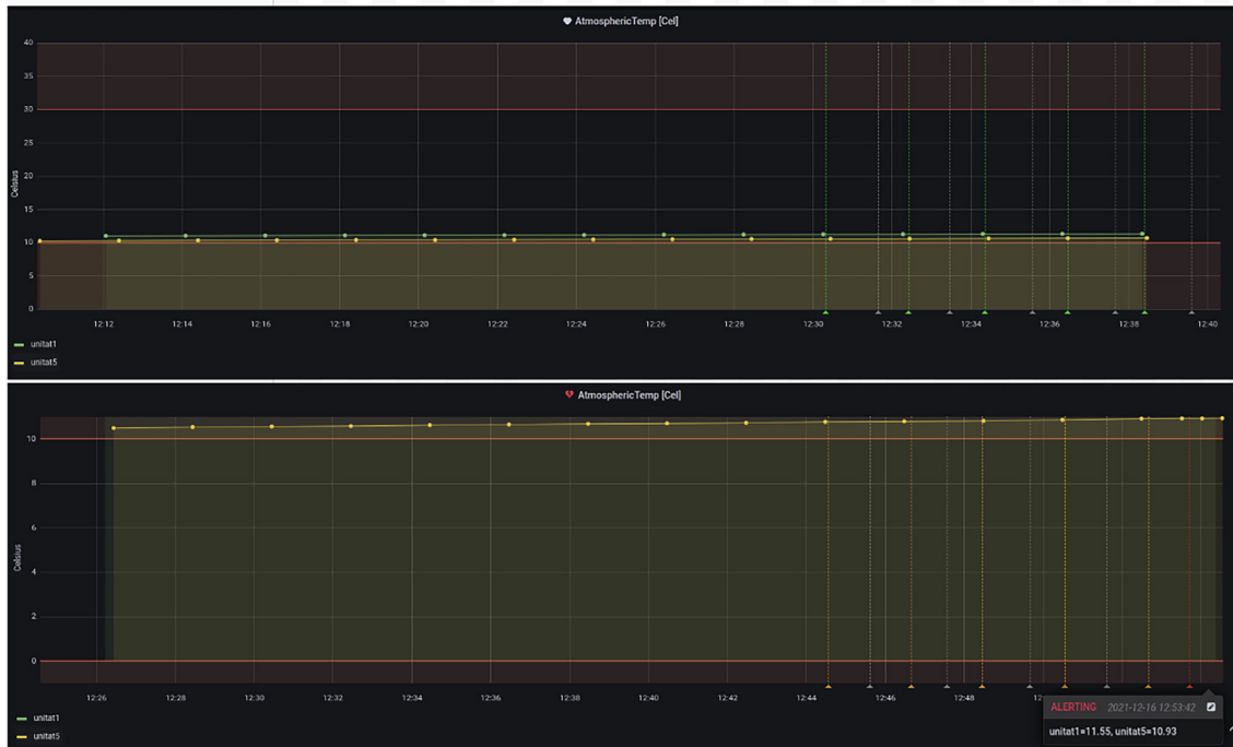
Fig. 12. System alerts: (top) sensor readings are within the user-defined range [10°–30°]; (bottom) sensor readings are outside the defined range [0°–10°] and are triggering the Alerting mode.
