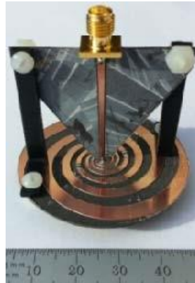
Figure 8: Constructed antenna and balun system (Jeon, Chang, & Pham, 2014)
