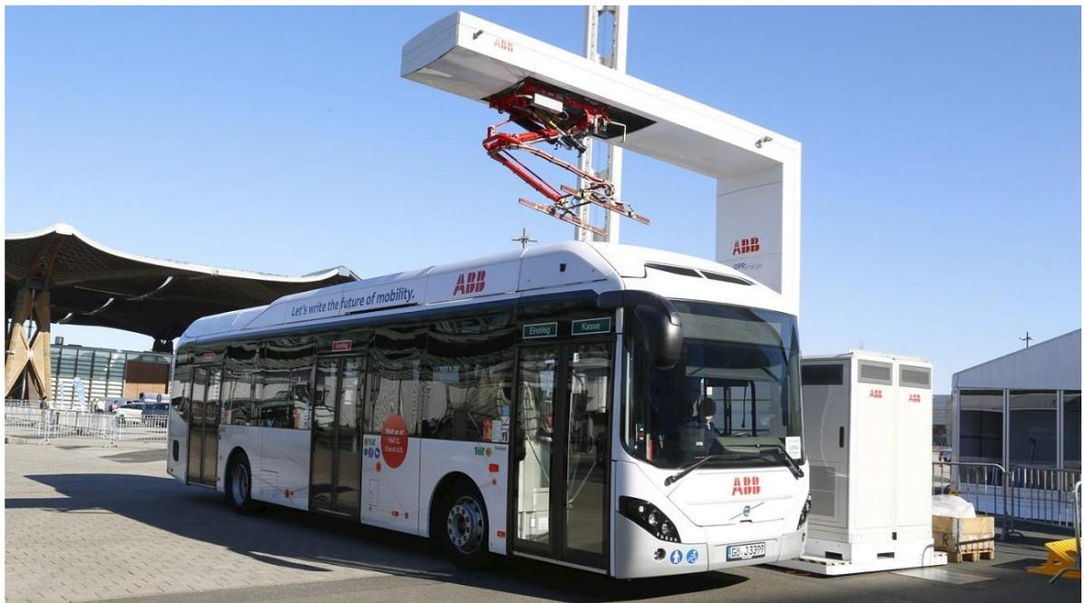
Figura 29: Sistema pantograph down de ABB [83]
