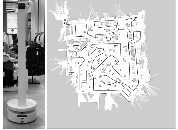
Fig. 4. The robot operating at the store (left), and the map of the store with the robot path containing the different aisles (right)
