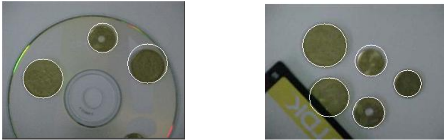
Figure 5. Two examples of counting coins. The white circumferences are the coins detected. Note that the CD is not detected as it has a different color, and the inner circle of several coins is not detected too.
