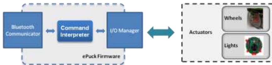
Figure 45: Conceptual map of the firmware
