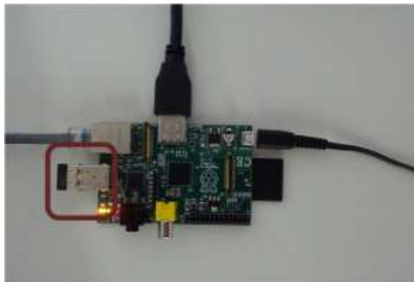
Figure 27: USB dongle used for Bluetooth communication (marked in Red)
