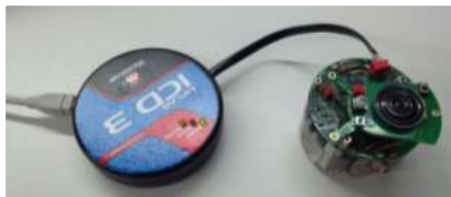
Figure 42: ICD3 programmer/debugger connected to E-Puck
