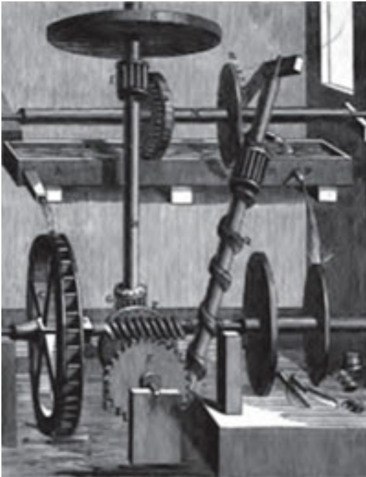
Figure 4. Example of inoperative device: perpetual motion machines
