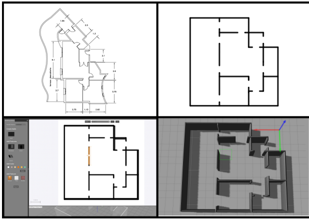
Fig. 3: Building a realistic map. Top row: Transform a real map to easy to reproduce one. Bottom row: Build the map and final result in the 3D simulator.
