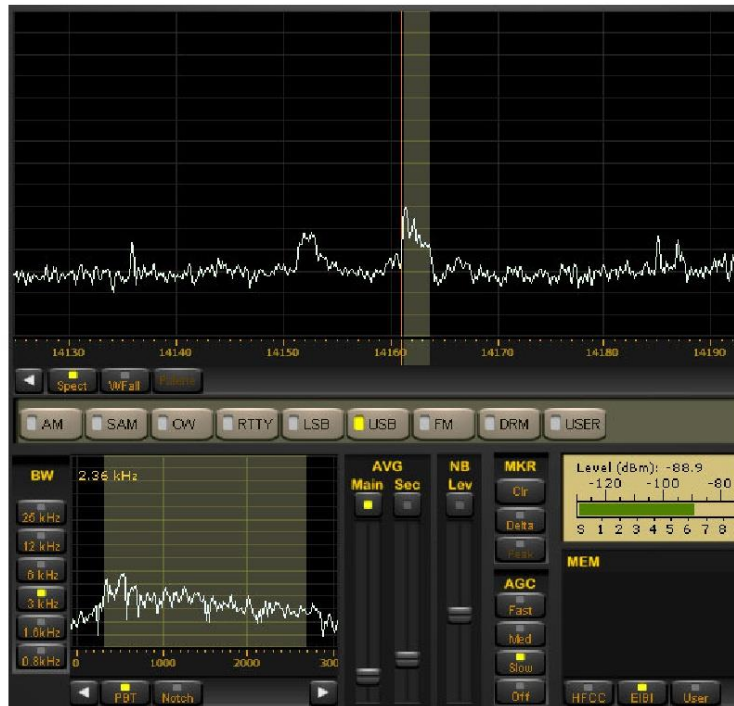
Dial pointer in spectrum mode in conjunction with the settings in BW pane
