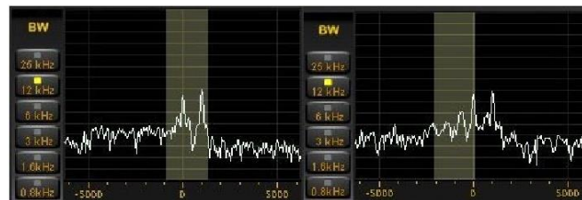
The freq centred on 1070 (left), but using PBT the QRM vanishes (right)
