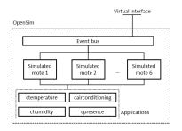
Applications developed in C as components of OpenWSN to simulate sensor data:
