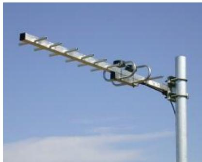
Figura 9 Antena Yagi
