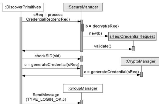
Figure 7: (Broker) Login sequence diagram: secureLogin function.
