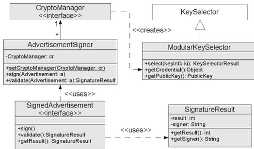
**Figure 9: Secure pipe advertisement class diagram detail with related classes.**
