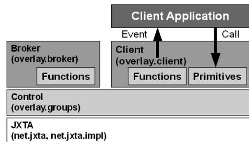
Figure 1: JXTA-Overlay architecture.
