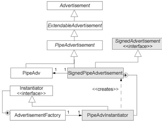
**Figure 8: Signed pipe advertisement class diagram with JXTA classes.**
