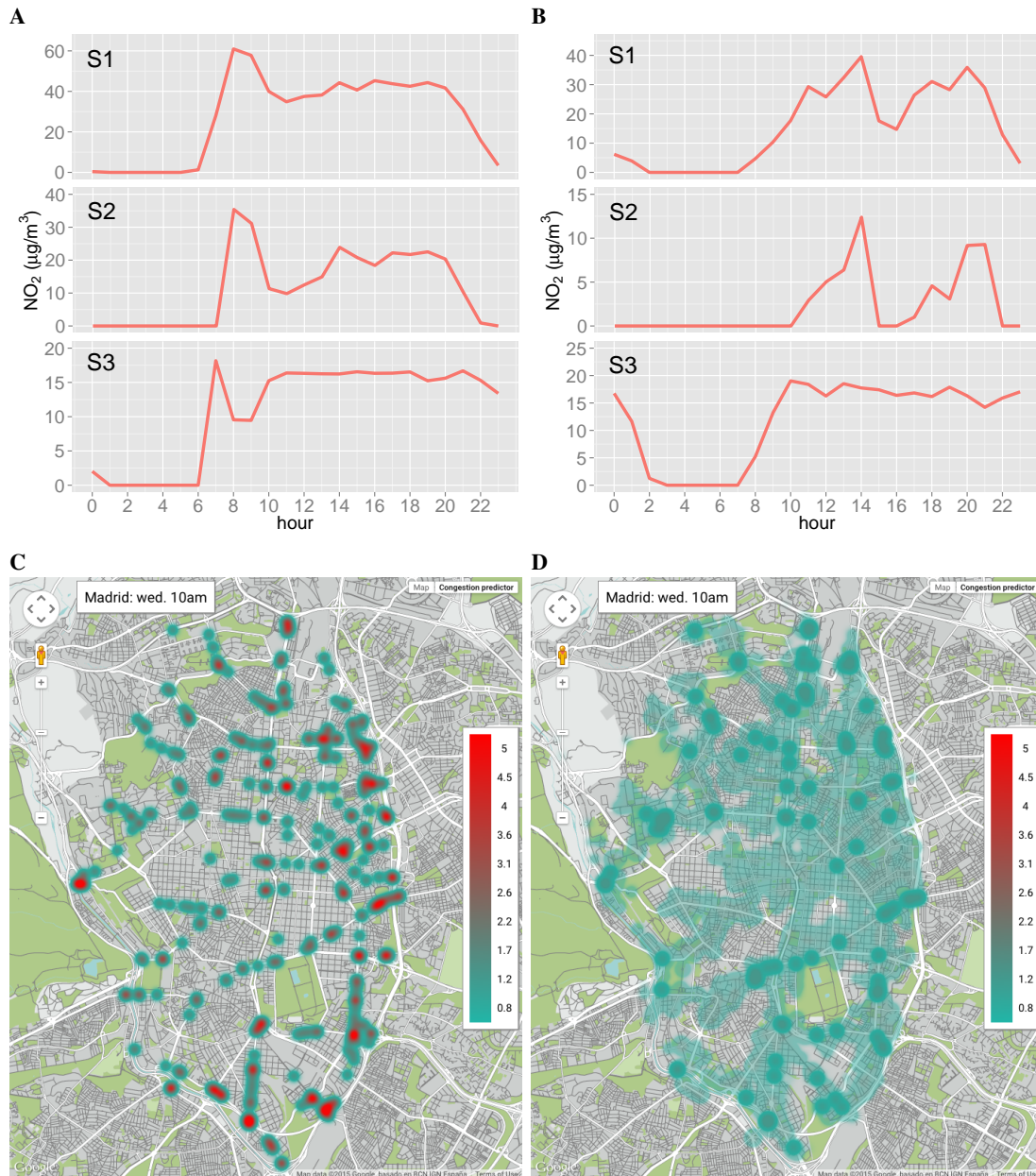
FIG. 10. Panels (A) and (B) show the expected decrement of NO 2 concentration for S1, S2 and S3 stations. Plots consider data from Monday to Friday (A) and weekend (B) and are grouped by hour of the day. Circles colored with green in Fig. 8 indicate the locations of S1, S2 and S3 stations. (C) Map of Madrid showing the ratio between incoming and outgoing vehicles for each congested junction before the establishment of the hotspot pricing scheme. Junctions with a ratio greater than 1 are congested since they receive more vehicles than the ones they can route. (D) Ratio between incoming and outgoing vehicles for the same junctions shown in (C) after the establishment of the hotspot pricing scheme.
